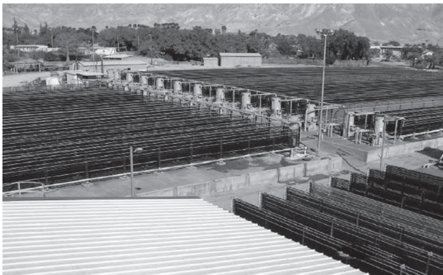
Fig. 1 An overview of tubular photobioreactors at Algatechnology's site for the production of astaxanthin rich Haematococcus biomass
